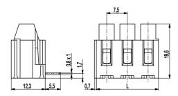
The PCB connector 152-A-111 is the horizontal version of 152-A-111 with a pitch of 7,5 mm is available with 2 or 3 poles.
