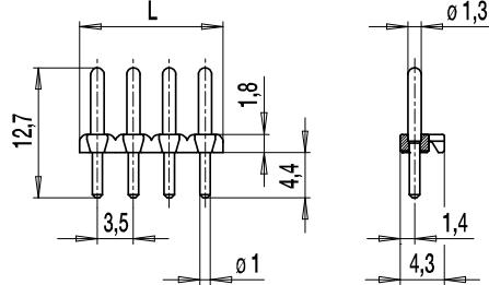
The pin strip 931-SLS features a pin diameter of 1,3 mm in the plug-in area and 1,0 mm in soldering area. When using with plug connector 938-FLDS, the housing extensions prevent incorrect plugging.
