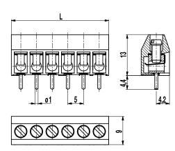
The PCB screw connector 970 with a pitch of 5 mm is available in 2- to 32-pole design
