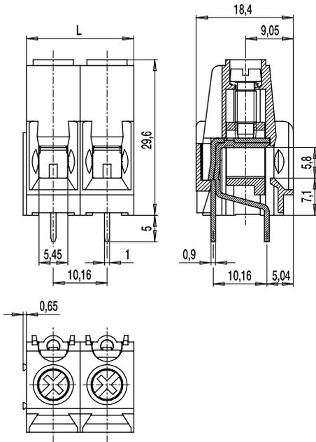
Series 158-A is particularly designed for high voltages and strong currents. A terminal space for solid wires of up to 16 mm<sup>2</sup> or for flexible wires of up to 10 mm<sup>2</sup> is characteristic for this series. Two solder pins per pole ensure safe connection to the PCB.
