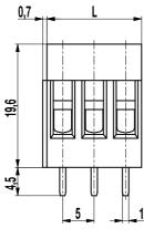
The PCB connector 150-A-111 with a pitch of 5 mm is available with 2 or 3 poles.
