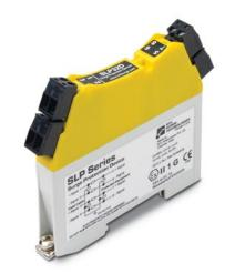
The multi-stage hybrid surge protection network at the heart of the SLP uses a combination of solid state electronics and a gas filled discharge tube (GDT) to provide surge protection up to 20kA. This impressive surge protection circuit is designed to exhibit exceptionally low line resistance and adds only a minimal voltage drop to the circuit.
