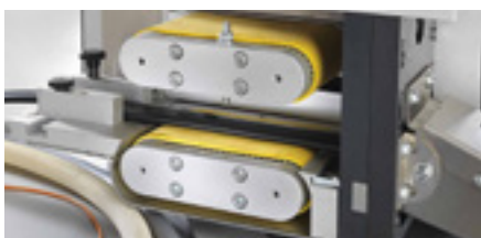
Universal transport unit for ribbon cables, round cables, insulating tubes and hoses
