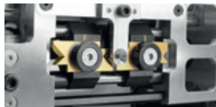
Stripping blade that can be used on both sides – for consistently high quality
