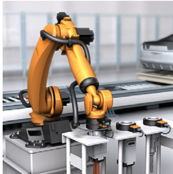
Industrial robots often perform several hundred tool changes per day. In this regard, conventional contacts are subjected to high levels of wear. With FreeCon Contactless, you benefit from a reliable and maintenance-free connection.
