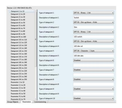
configured. The KNX data point type has to be set and group addresses have to be assigned. To simplify this task for each KNX BAOS Module or Device a corresponding ETS product entry is available from the Weinzierl website.
