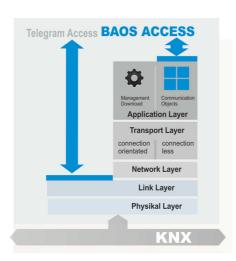
The KNX system itself is a decentralized network and the runtime communication is based on group telegrams in multicast. To participate in the KNX runtime communication each device must be configured, e.g. group addresses must be assigned. Typically this is done via the ETS<sup>®</sup> (Engineering Tool Software) program, the official tool available from the KNX Association. The configuration can be loaded into the distributed devices via the KNX network
