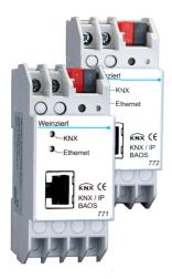
Using the KNX IP BAOS 771, 772 or 777 the KNX bus is accessible from everywhere via Ethernet. Connection over WiFi (with an extra router) or the Internet is possible, too. The IP settings as well as the data points can be configured with ETS software. The device requires either an external power supply or via Power-over-Ethernet (IEEE 802.3af) directly from the switch. This device can be also be used as a programming interface for ETS.
