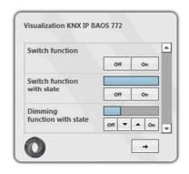
To demonstrate the KNX BAOS architecture the KNX BAOS Gadget has been created as a sample. It shows the possibilities to configure even complex applications like visualizations just using ETS parameters.
