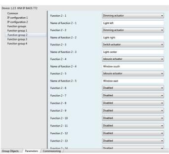
Plug-In or editor is not required. The configuration is done only via the ETS parameters of the KNX IP BAOS 772 using the product database with building structure. The rooms and functions can be arranged very simply and can be denoted with any text you like. The appropriate communication objects are displayed automatically and can be linked with
