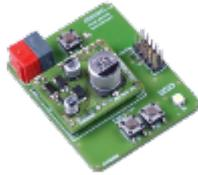
The *Demonstration Board* is a simple board which demonstrates the usage of KNX by switching or dimming a LED with two buttons. For development projects we recommend the Development Board. (See [Chapter 3, The Development Board](#))
