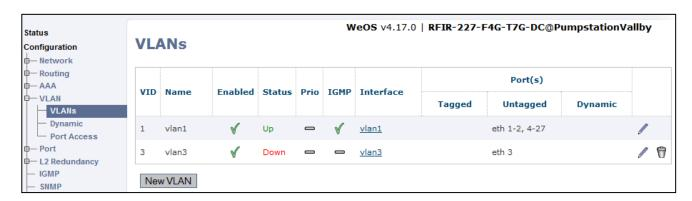
2. Then setup IP-addresses to turn the VLANs into layer 3 interfaces. Configuration -> Network -> Interface.
