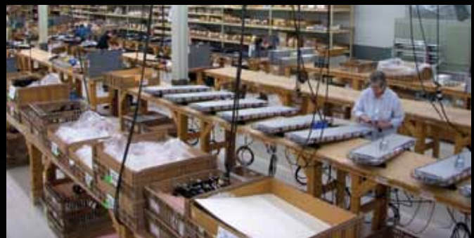
Lightbar Final Assembly
