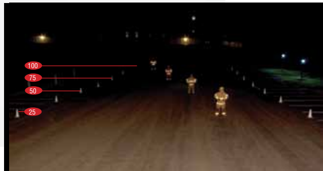
Quartz Halogen Single Lamp (300w - 24amp)
