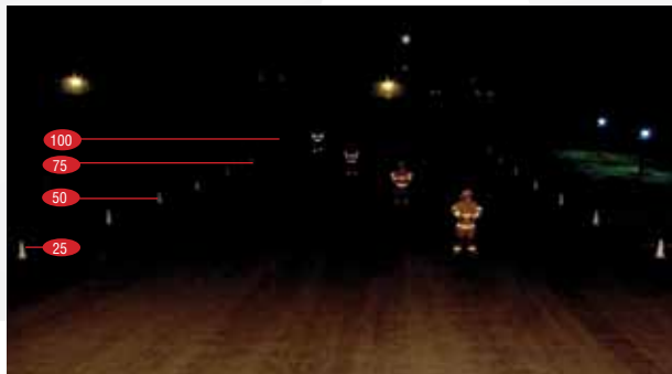
Quartz Halogen Single Lamp (150w - 13amp)
