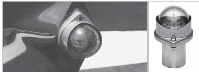
2. This unit fits directly in place of the Grimes Model S tail position light. It is however sometimes necessary to open the mounting hole in the aircraft fairing to 1.10 inch, to clear the body of the A500A. The body protrudes 1.40 inch into the tail fairing.
