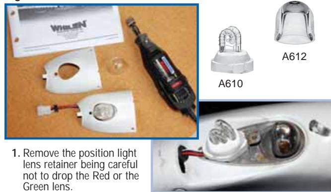
1. Remove the position light lens retainer being careful not to drop the Red or the Green lens.
