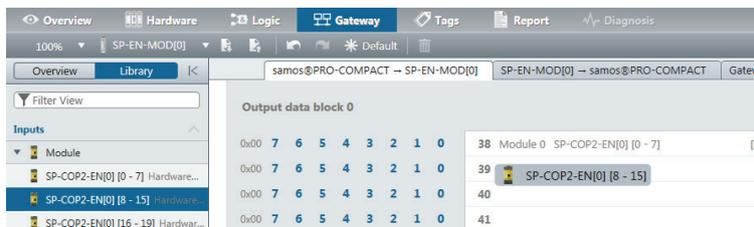
Illustration 8: Use drag&drop to move the data bytes to the routing table.
