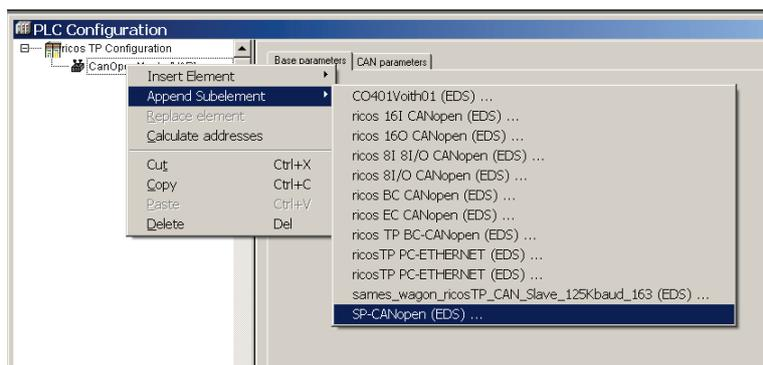
Illustration 51: Attaching the SP-CANopen with CoDeSys 2.3
