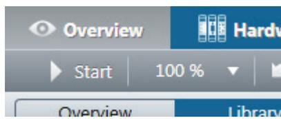
Illustration 23: "Start" button indicating device is not in "Run" mode
