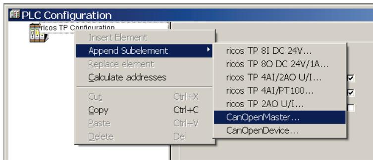
Illustration 50: Attaching a CanMaster with CoDeSys 2.3
