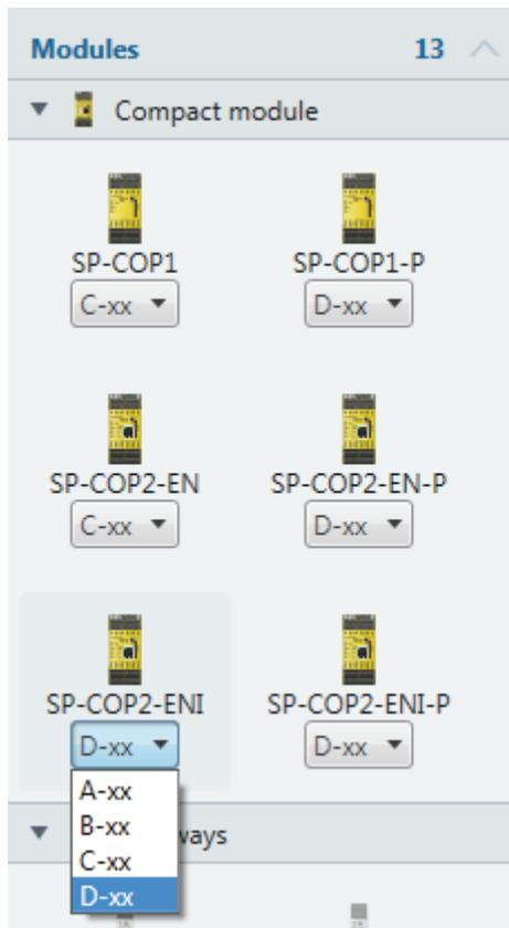
Illustration 21: Selection of module type for EtherNet/IP in samosPLAN5+
