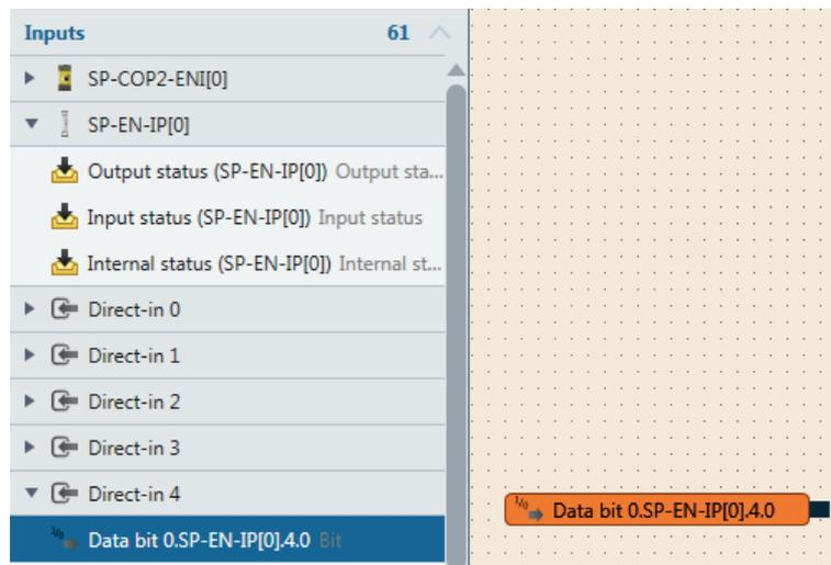
Illustration 27: Adding gateway data elements via Drag'n'Drop in the logic editor of samosPLAN5+
