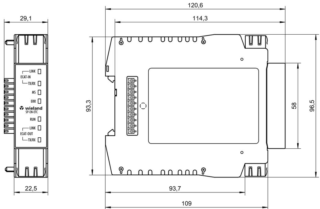
Illustration 65: Dimension drawing of EtherCAT gateway SP-EN-ETC (mm)
