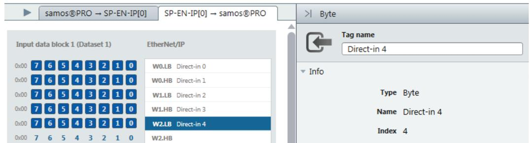
Illustration 26: Adding new data byte (O→T) for use in the logic editor by configuring the tag name.
