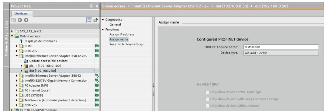
Illustration 13: Assigning device names with the TIA portal
