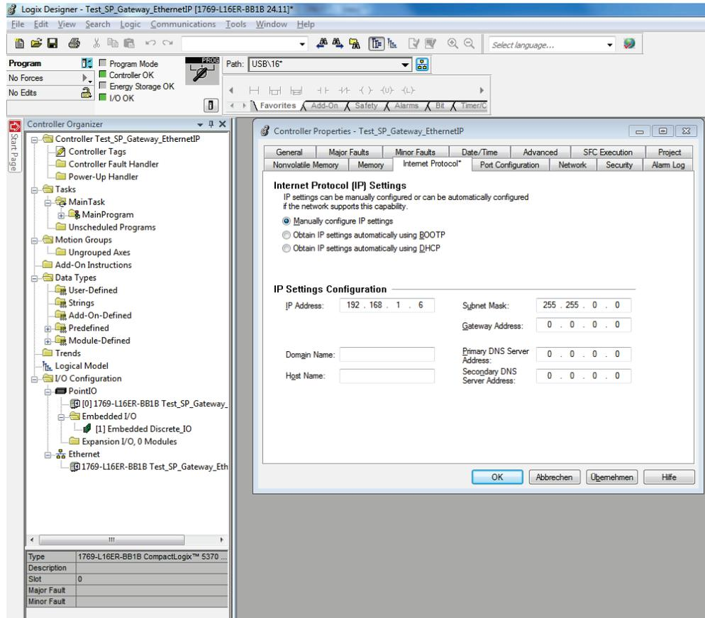
Illustration 18: IPv4 setup for device in Logix Designer
