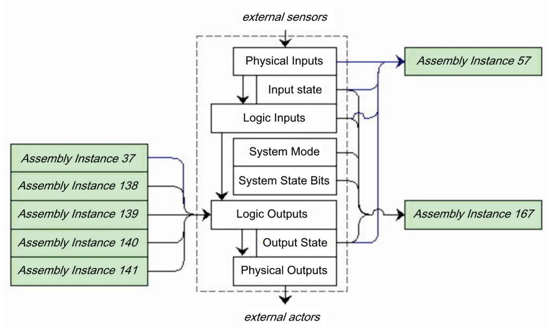
Illustration 31: Data flow with usage of Assembly Instances provides by SP-COP2-ENI
