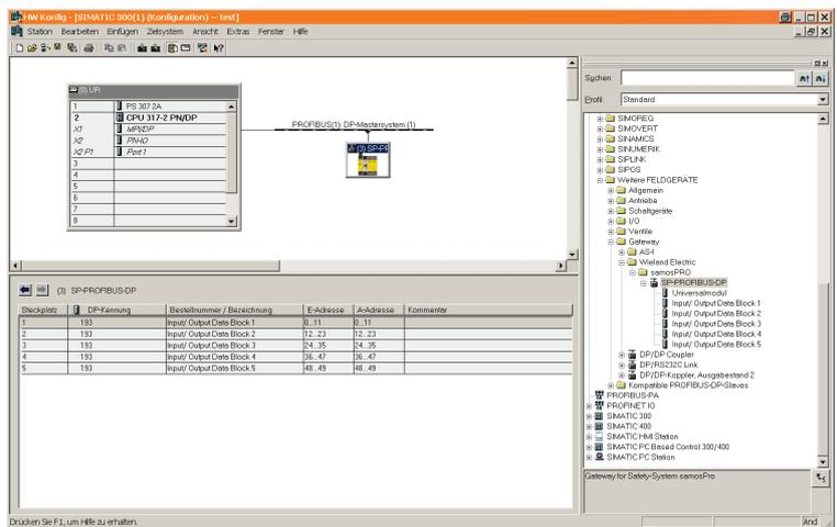
Illustration 38: Example for a PROFIBUS-DP configuration in the Siemens SIMATIC manager
