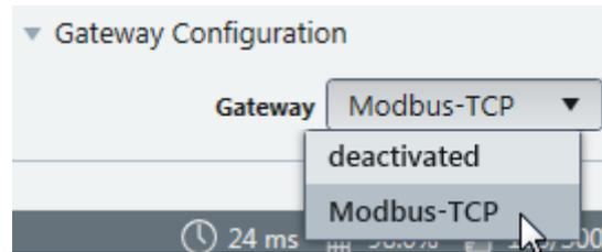
Illustration 11: Activation of Modbus TCP on the SP-COP2-ENI module
