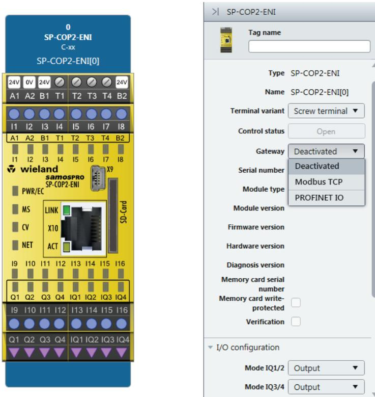
Illustration 2: "SP-COP-ENI" module with activated gateway function
