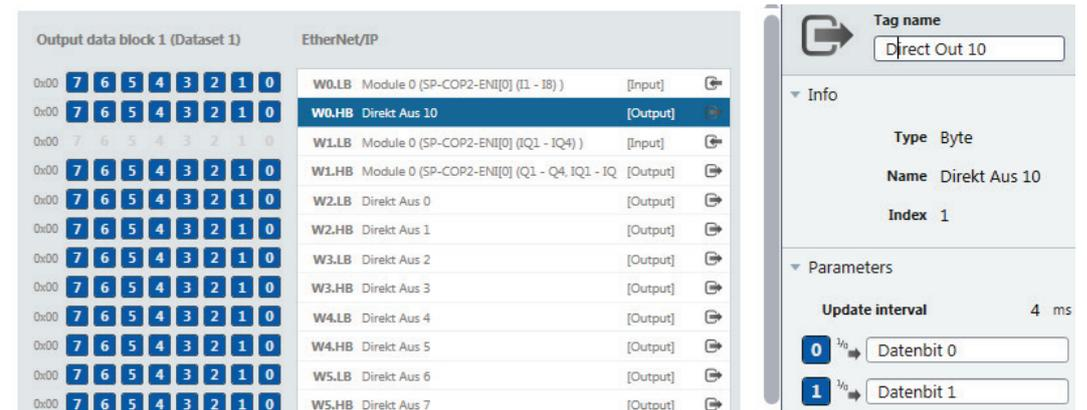
Illustration 25: Adding new data bytes (T→O) for use in the logic editor by configuring the tag names
