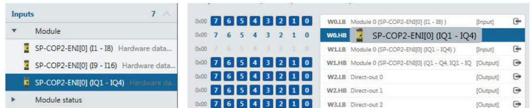
Illustration 24: Adding bytes into the gateway process data image (T→O) via Drag'n' Drop in samosPLAN5+
