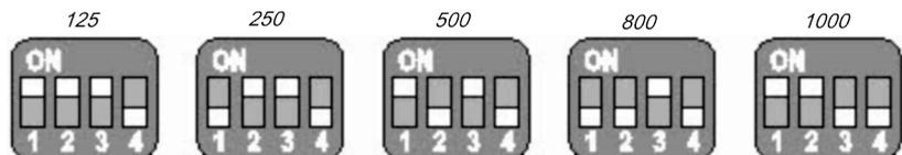
Illustration 46: Setting the DIP switches on the SP-CANopen
