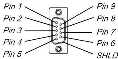
Illustration 36: Pin configuration of D-sub socket and plug for the SP-PROFIBUS-DP
