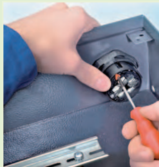
Fasten or loosen the contact insert
