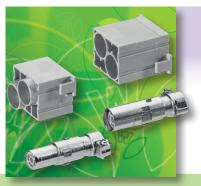
The modular **revos**FLEX system is being expanded by TWIN BUS inserts. They are extremely suitable for transferring sensitive signals in heavy-duty plug connectors. The contact carrier is designed for two plug inserts. The connection system is achieved via the tried and proven turned  $\emptyset$  1.6 mm contacts, and offers a connection range of 0.5-2.5mm² with a rated voltage of 50 V and a rated current of up to 10 A.
