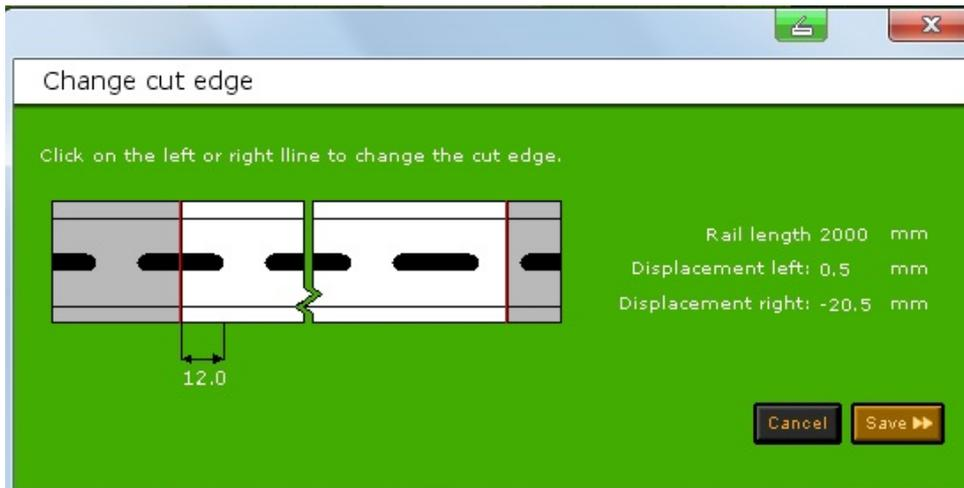
The two red lines show the original cutting edge. With the mouse you can now move the left and/or the right cutting edge as you like. Take over the chosen adjustment via the "Save" button. When you move the left cutting edge, the total rail length remains constant. The right cutting edge allows you to modify the rail length as you like.
