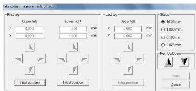
engraving arm now moves to the upper left corner of the engraving field. You can use the relevant cursor buttons as shown to move to the exact position of the upper left corner for the first tag.
