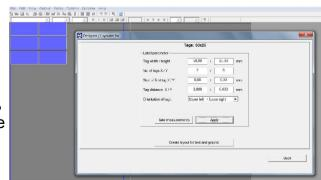
To measure using the plotter, all you have to enter is the number of tags along the X- and Y-axes. All the other data can be easily calculated using the program and with the help of the plotter.
