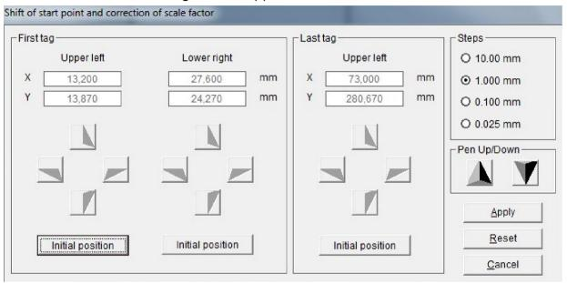
Insert a plotter pen into the pen holder and click on the button **Initial Position** in the far left field.
