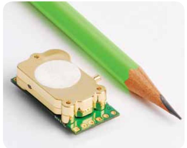
The Telaire<sup>®</sup> T6703 CO<sub>2</sub> Series is ideal for applications where CO<sub>2</sub> levels need to be measured to make assessment of indoor air quality.
