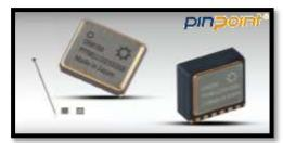
PinPoint® is a tiny (6.3x5.5x2.7mm), yet powerful, surface mountable LCC ceramic packaged, single-axis MEMS angular rate sensor (gyro), capable of measuring angular velocity up to a maximum of ±1,000% which has two output modes; an analogue voltage signal which is linearly proportional to angular speed, and a digital signal in SPI® protocol. The choice of output mode; analogue or digital, is determined by the user when connecting it to the user's host PCB.
