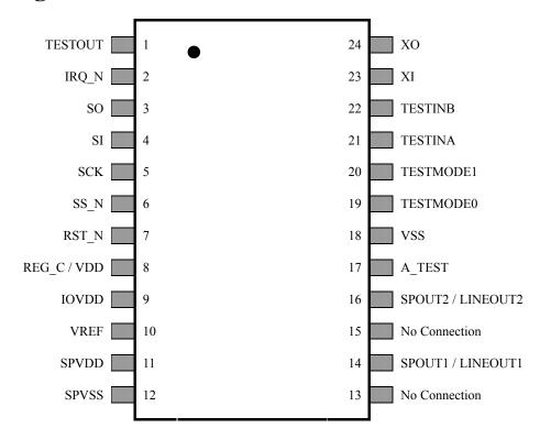
24-pin SSOP TOP View
