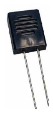
Amphenol's Thermometrics HS12SP model is a nonrefresh type of polymer based relative humidity sensor
