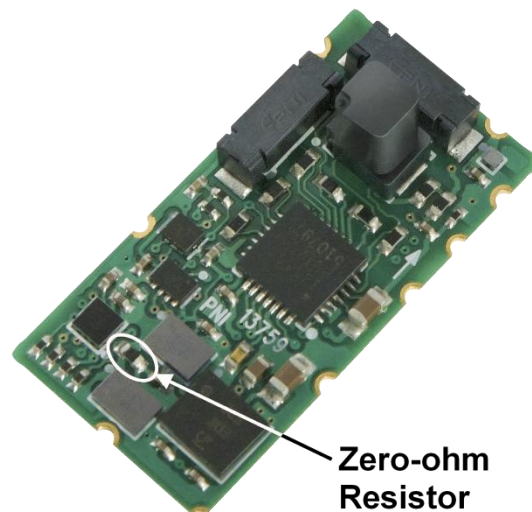
Figure A3-0-1: SENtral Blue M&M Zero-Ohm Resistor Location
