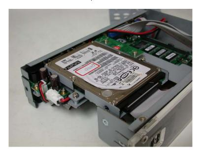
(3) Connect the 44-pin HDD cable to CON 11.
