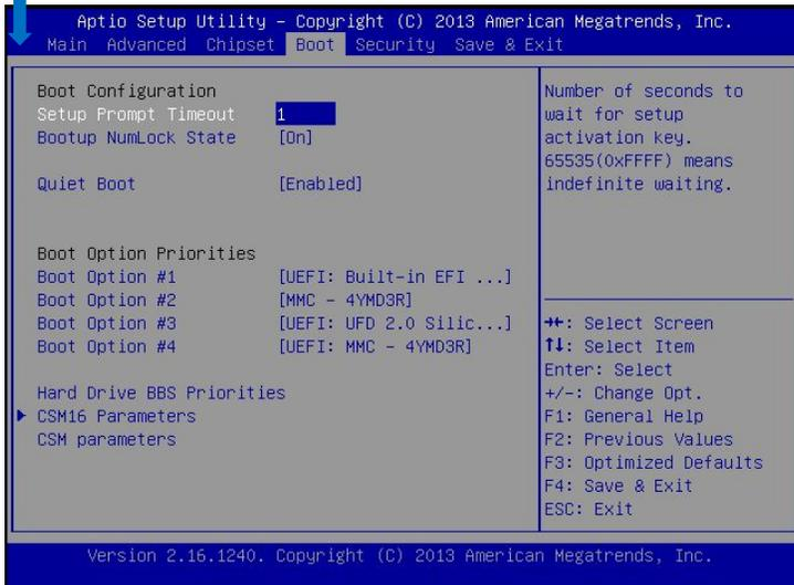
2. Move between items and select values by using the arrow keys. Modify the selected fields using the PnUP/PgDN Keys. For information on the various options, press <F1> key.
