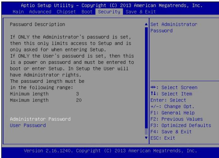
2. Move between items and select values by using the arrow keys. Modify the selected fields using the PgUP/PgDN keys. Please press the <F1> key for information on the various options.
