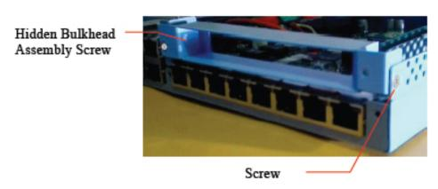
This retainer supports the chrome bulkhead bracket of standard PCIe cards. With the retainer removed from the chassis the hidden bulkhead assembly screw becomes visible. Remove the blank bulkhead bracket.
