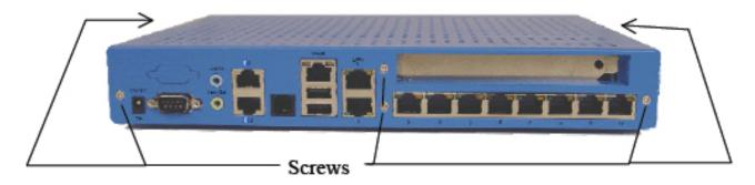
After removal of the fasteners the top cover slides back.
