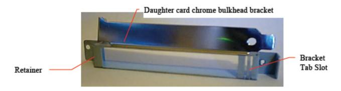
Seat the daughter card into the PCIe and/or the AUX connectors and reinstall the screw that holds the retainer to the chassis. Replace the top cover.
