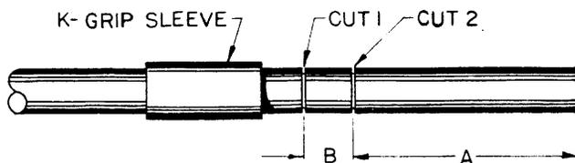
1. Cut cable end square, slide shrink tubing and K-grip sleeve over jacket and with jacket trim jig make cuts 1 and 2 in jacket.
