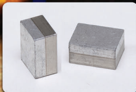
Explosively welded aluminum to stainless steel
