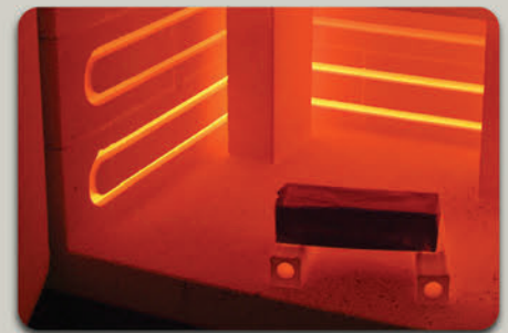
Composite metal sintering and densification
