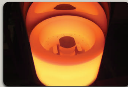
Vacuum Brazing copper to stainless steel
