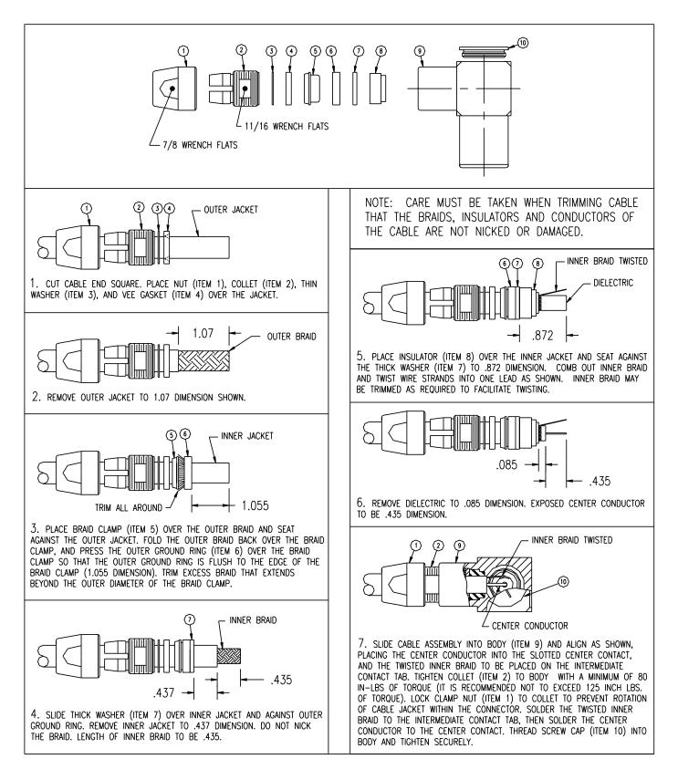
Crimp Dies are available for above operations. (See page 28 and 29 for part numbers.) Tri-Loc Inspection Gauges are available. (See page 37 for part numbers.) ALL DIMENSIONS ARE IN INCHES
