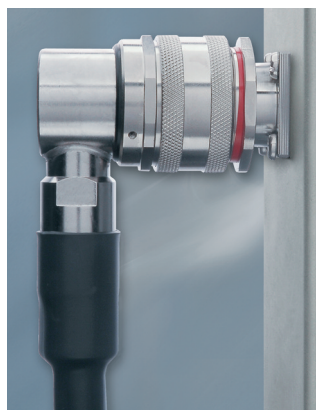
TRU-SQS® spring-loaded sleeve is retracted and interfaces engaged. Note TRU-Redline™ indicator is still visible until sleeve is released and a fully mated condition is present.
