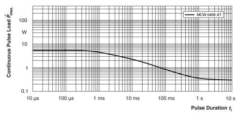
Maximum pulse load, continuous pulses; applicable if  $\bar{P} \leq P\left(\vartheta_{\text{amb}}\right)$  and  $\hat{U} \leq \hat{U}_{\text{max}}$ ; for permissible resistance change equivalent to 8000 h operation in standard operation mode
