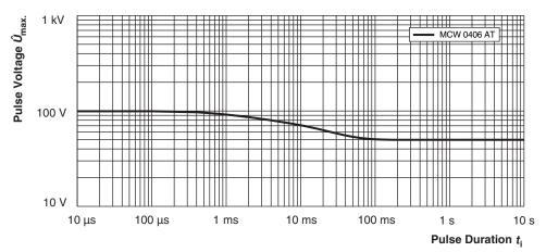
Maximum pulse voltage, single and continuous pulses; applicable if  $\hat{P} \leq \hat{P}_{\text{max.}}$ ; for permissible resistance change equivalent to 8000 h operation in standard operation mode
