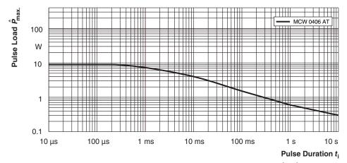
Maximum pulse load, single pulse; applicable if  $\bar{P} \to 0$  and  $n \le 1000$  and  $\hat{U} \le \hat{U}_{max}$ ; for permissible resistance change equivalent to 8000 h operation in standard operation mode
