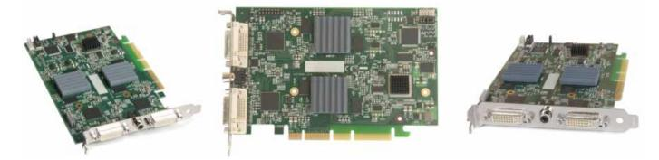
XV-AVHD has three independent video capture inputs - two supporting HD capture and a third supporting SD composite video. The XV-AVHD also adds multiple channels of audio capture, which can be synchronised in software using time stamping with all video capture channels.
