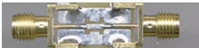
Figure 2. Example microstrip test fixture.
