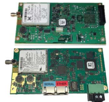
Xeta9x Emancipator Series 902-928 MHz Serial/Ethernet Up to 2.6 Mbps
