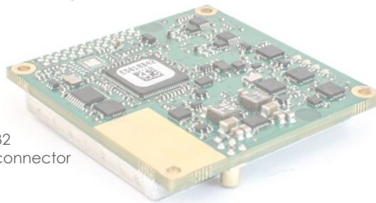
Dimensions (L x W x H) 2.0 " x 2.0 " x 0.37 " / 5.1 cm x 5.1 cm x 0.94 cm Weight 0.06 lbs / 30 grams
