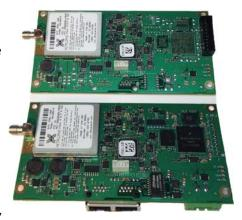
power output from 10mW to 0.61W, and channel sizing from 12.5 kHz to 50 kHz. The **Xeta14x** selectively switches modulation schemes to ensure required throughput given available channel sizes and environmental noise. Based on its patent pending Dual Decode Digital Architecture<sup>™</sup>, XetaWave's technology platform offers performance second to none in the commercial market today.
