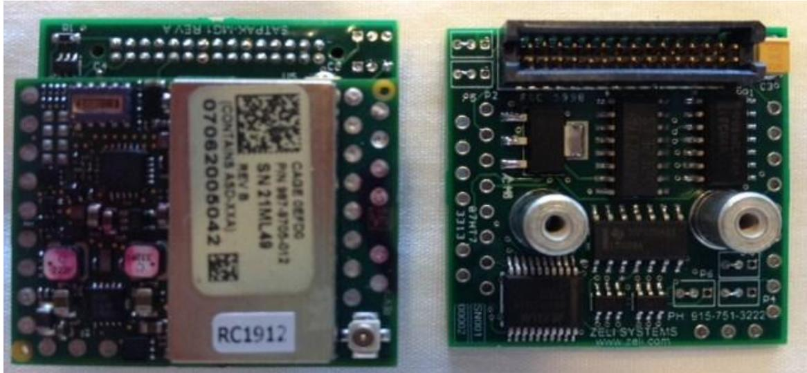
**MicroGRAM Attached to Component Side of SATPAK-MG**
