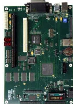
The design is available at no cost and may be used as is or modified to suit specific needs. The [design package](#), available from ZF, includes [OrCad schematic](#), PadsPCB Layout files, and a complete Bill of Materials spreadsheet. Included with the ZFx86 System-On-Chip are a [ZF BIOS](#) (based on Phoenix Technologies kernel), DR-DOS 7.03 license, and software drivers to support all hardware. Additionally, Windows CE® and Linux are available and ready to run.
