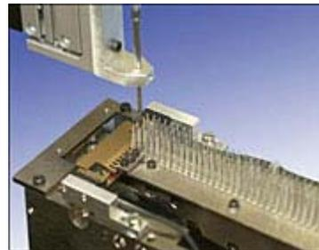
Feeder capacity is 24" of the header strips. New strips can be loaded on the rear of the feeder at any time as long as there is room for the strip. At the pick point, the first header is separated from the strip and presented for pickup. Sensors on the cylinders provide feedback to the microprocessor for control purposes. LEDs on the microprocessor PCB provide the status of all sensors.
