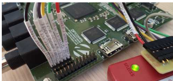
Figure 17: FPGA programming set-up using the JTAG header
