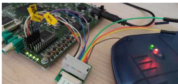
Figure 18: ATmega programming set-up using the JTAG header
