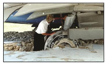
EMASMAX is a bed of customized cellular cement material, designed to crush under the weight of an aircraft, thus providing predictable, controlled deceleration. Once stopped, EMASMAX's unique material allows passengers and crew members to exit the aircraft safely and for the aircraft to be easily removed from the arresting system.
