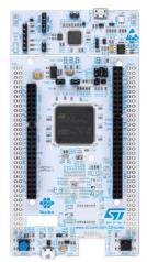
Top view of a NUCLEO-FXXXZY board without Ethernet peripheral.
