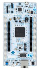
Top view of a NUCLEO-FXXXZY board with Ethernet peripheral.
