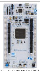
Top view of a NUCLEO-L4XXZY board without Ethernet peripheral.
