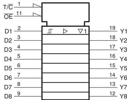
**LOGIC DIAGRAM (POSITIVE LOGIC)**
