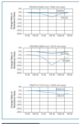
Anti-Surge Thick Film Chip Resistors(ERJP Type) Thick Film Chip Resistors(ERJ Type)
