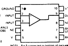
NOTE Pin 5 connected to bottom of package
