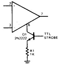
INCREASING INPUT STAGE SLEW RATE\*
