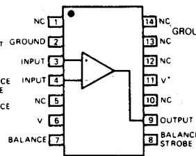
NOTE Pin 6 connected to bottom of package
