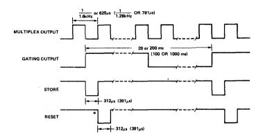
Referring to the test circuit, the crystal oscillator frequency is divided by 2<sup>12</sup> to provide both the multiplex frequency and generate the output pulse widths. The GATING OUTPUT
