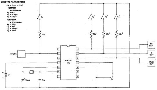
SWITCHES  $\mathbf{s}_1, \mathbf{s}_2, \mathbf{s}_3, \mathbf{s}_4$  OPEN CIRCUIT FOR SUPPLY CURRENT MEASUREMENT. SWITCH  $\mathbf{s}_5$  OPEN CIRCUIT FOR SLOW GATING PERIOD.
