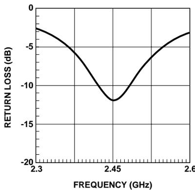
**Figure 18. Input Return Loss, 3  $\mu$ A Bias.**
