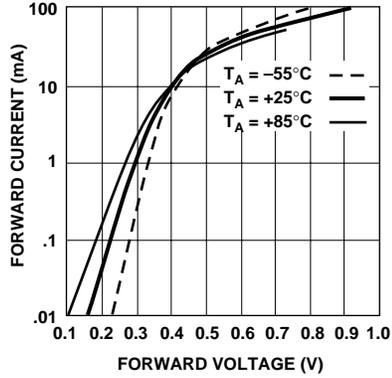
Figure 1. Forward Current vs. Forward Voltage at Temperature.
