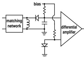
Figure 27. Differential Detector.
