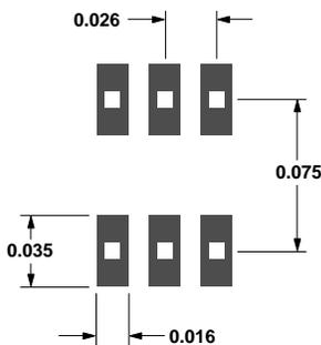
Figure 34. PCB Pad Layout (dimensions in inches).
