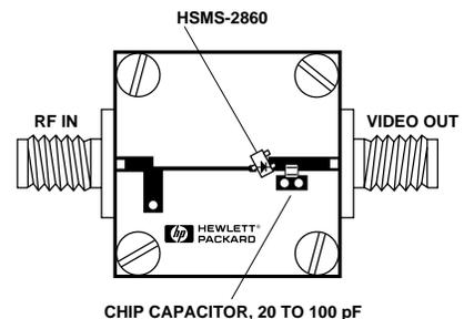
Figure 16. Test Detector.
