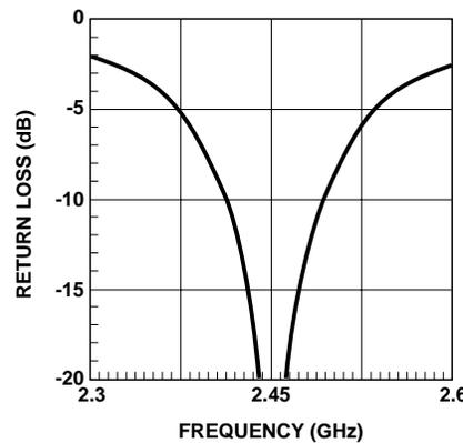
**Figure 20. Input Return Loss. Modified 2.45 GHz Circuit.**
