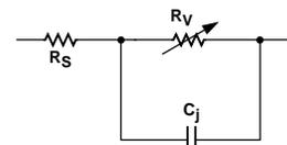
Figure 8. Equivalent Circuit of a Schottky Diode Chip.
