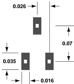
Figure 33. PCB Pad Layout (dimensions in inches).
