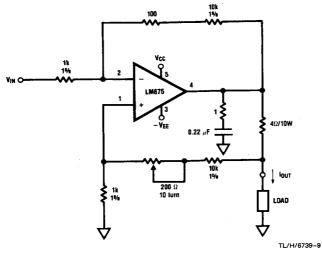
$i_{OUT} = V_{IN} \times$  2.5 amps/volt i.e.  $i_{OUT} =$  1A when  $V_{IN} =$  400 mV
