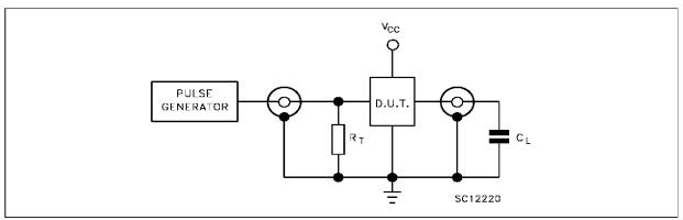
$C_L = 15/50 \text{ pF}$  or equivalent (includes jig and probe capacitance)
